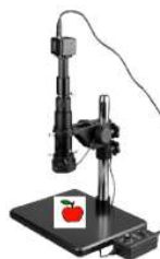
Figure 3. The camera is statically mounted for fruit grading and sorting
